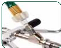
4. Slowly turn on the water. The water should come out of the front QC coupler. If it does, proceed to section B.
