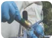
4. Slowly turn on the water supply and allow the water to flush the injection unit.
